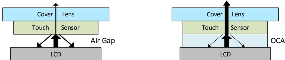
*A significant portion of the backlight is internally reflected within the air gap layer.*
