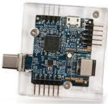
It also has a USB Micro-B port for connecting to a computer running the EZ-PD analyzer software. The software shows every PD message and acknowledgment exchanged between the two devices. It also shows the VBUS voltage and current:
