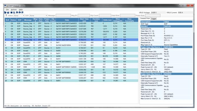
The EZ-PD Analyzer is an inexpensive tool for monitoring USB-C PD negotiations, voltage, and current during development.
