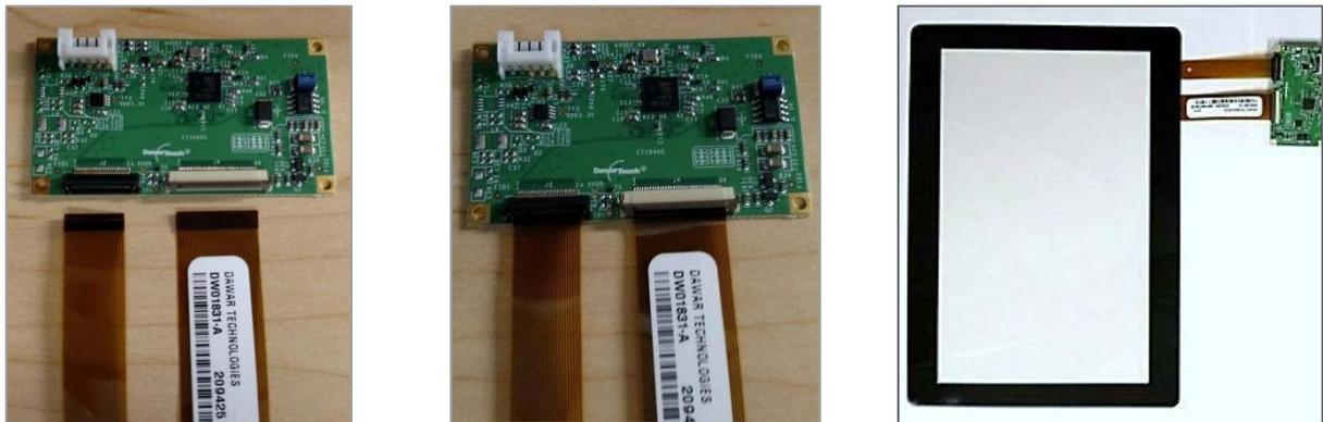
Note that the location of the controller board may be different than shown above. The touch sensor will only plug into the controller board in one direction.
