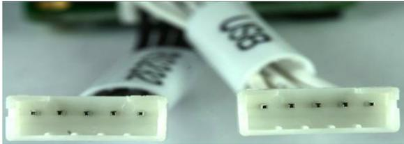
This cable has a total of 3 connectors: one connection to the controller board and two connections to either USB or Serial cable.
