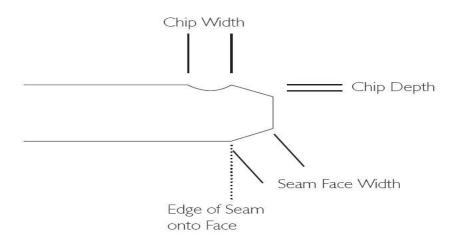
Chip width is measured from the edge of the seam on the face; chip length is the distance along the edge. Chip depth typically should not exceed  $\frac{1}{2}$  the thickness of the part.
